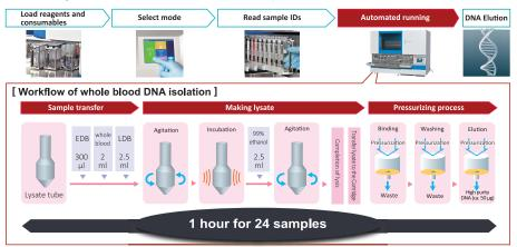
Max. 24 samples in a single run with the process time in 1hour.
