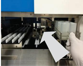
(4) Set wash buffer bottle in the wash buffer bottle rack in the drawer (at setting position No.4).
