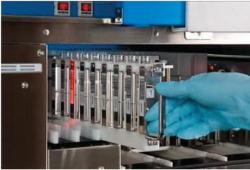
(A-2) Insert sample holder A in slot A slowly over approx. 8 seconds. The ID is read. Securely set until it contacts the stopper on the end.
