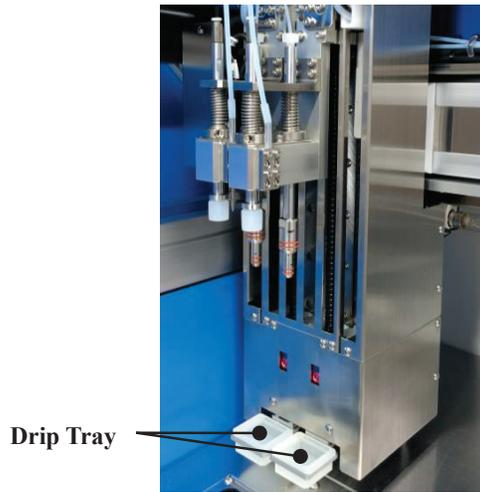
Drip trays are mounted on lower part of robot unit.
