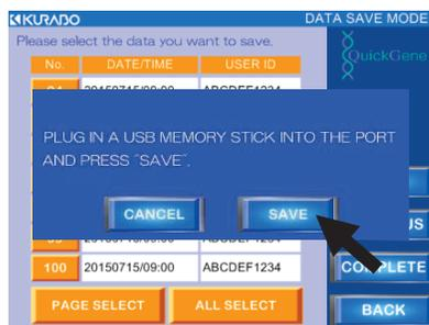
(6) When pop-up window is displayed, insert USB memory stick in USB port on side surface of system. Then press [SAVE] in pop-up window.
