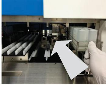
(4) Set wash buffer bottle in wash buffer bottle rack in drawer (at setting position No.4).
