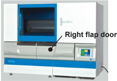
(A-1) When the door lock is released, open the right flap door.
