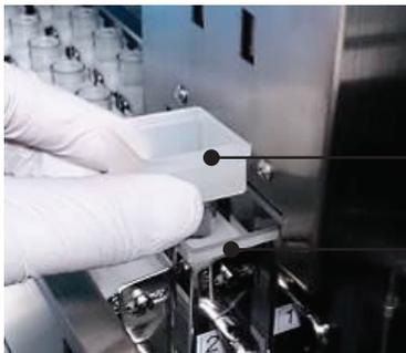
(5) Mount cleaned or new drip trays on drip tray guide.
