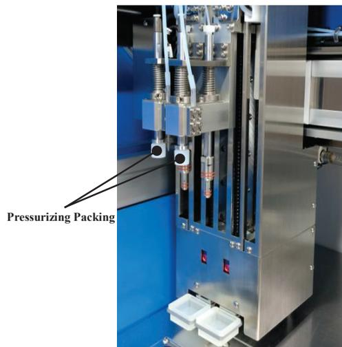
Pressurizing nozzle (packing) is mounted on robot unit.
