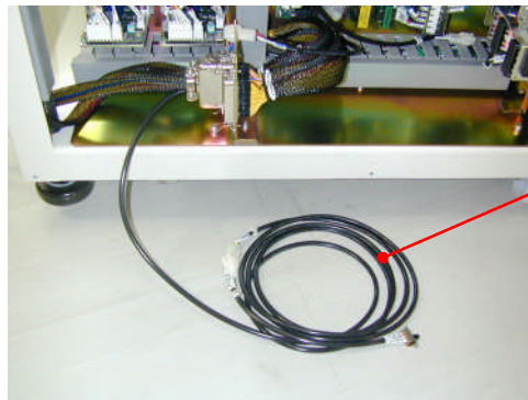
Three/six optional dispenser channel changing switch cable
